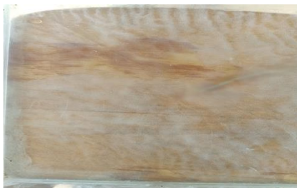
Figure 28, the Precipitated salt due to Alum reaction
